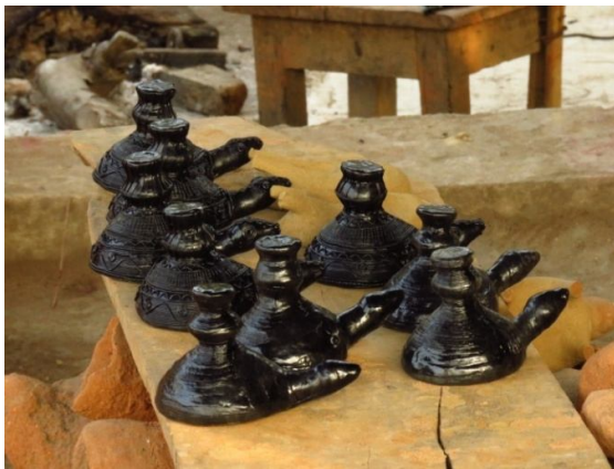
Wax moulds before clay plastering being kept
