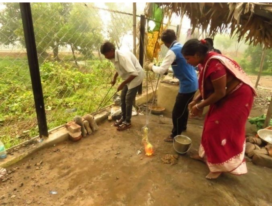
The fired moulds being taken out of the hearth
